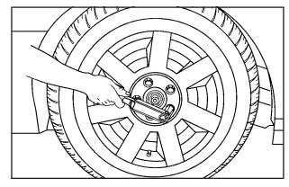
2. For models with exposed lug nuts, loosen them using the wheel wrench. Do not remove them yet.
